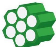
Figure 1. NSBA-15 having mesoporous 2D hexagonal structure
