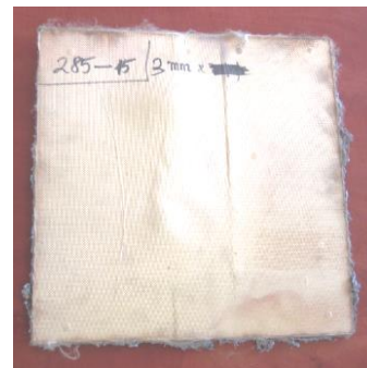
Figure 4. Ballistic protection plate rear side (after firing)
