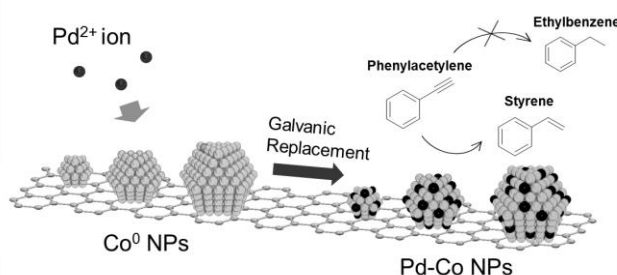
Figure 1 Structural transformation from Co NPs to Pd-Co NPs by galvanic replacement method.
