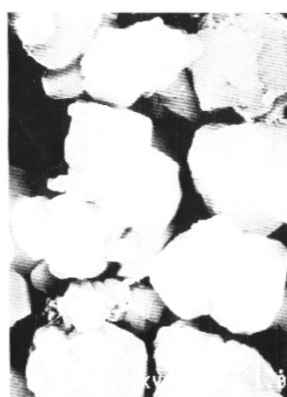
Products of 1970's \text{SiO}_2/\text{Al}_2\text{O}_3 = 4.8
